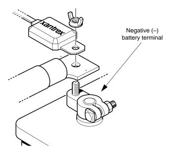
Figure 7 BTS Mounted on the Negative Battery Terminal
